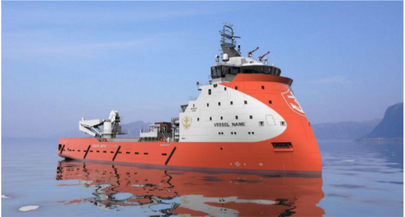
Illustration with crane and ROV (preparations only)
